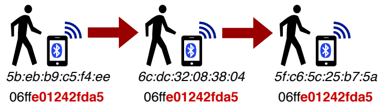
Figure III.1 – Representation of a successful attack. The BLE device is randomizing its BD_ADDR (in italic ) over time while keeping a static identifier (in bold ) in the advertising data. Such a 5-byte identifier can be used by a passive attacker to link together the packets generated with the three different BD_ADDR.
