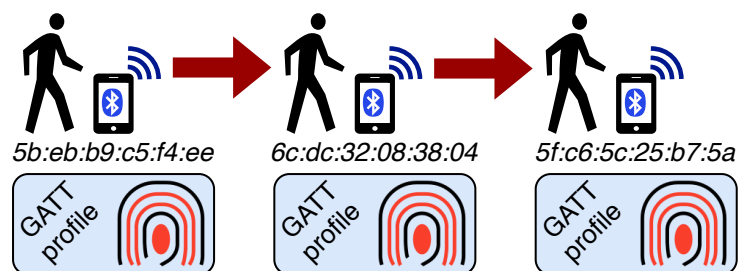
Figure III.12 – Representation of a successful attack. The BLE device is randomizing its BD_ADDR (in italic ) over time while keeping a static GATT profile. Such a GATT profile can be leveraged by an active attacker to generate a fingerprint of the device before to link together its three different BD_ADDR.
