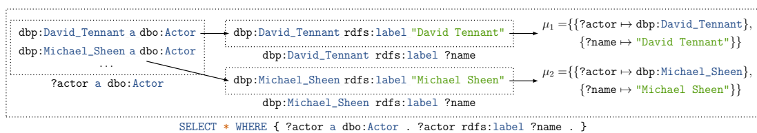
Figure 2.11: Basic Graph Pattern evaluation using the TPF Smart client [72]
