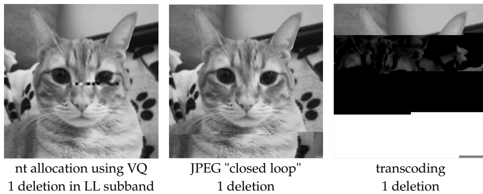
Figure 5.7: The impact of one deletion error on a 512x512 pixel image of a cat for the different encoding solutions. The original images have been compressed to obtain the same PSNR value of 38.5 dB.
