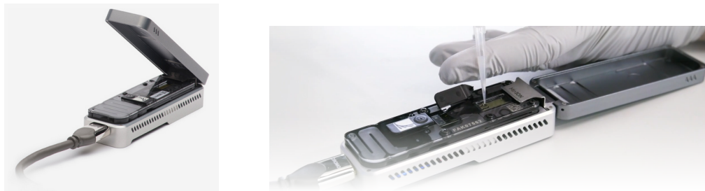
Figure 2.10: The MinION nanopore sequencer by Oxford Nanopore Technologies 2
