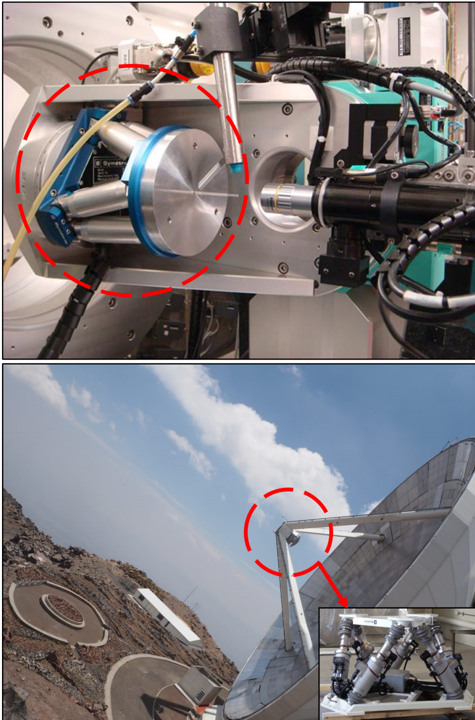
Figure 4: Figures showing hexapods used for high-precision 6-DOF positioning applications such as for positioning samples in synchrotrons [Symétrie, c] (top) and for positioning mirrors in telescopes [Symétrie, e] (bottom)
