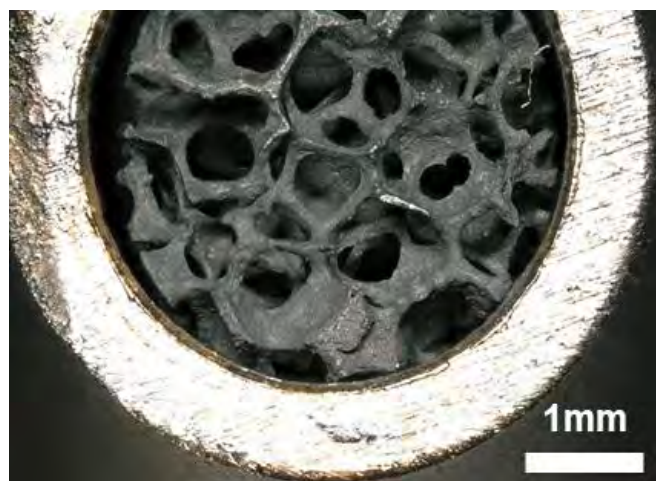
Figure 4.25. Photo of the metallic foam coated in the tubular reactor for catalyst stability study under continuous reactor operation.
