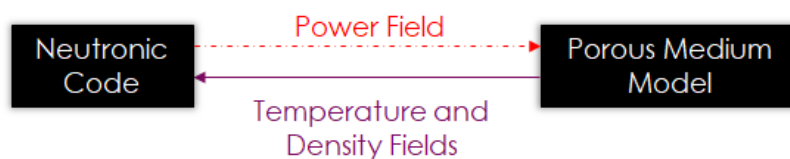
FIGURE 5.28 – Neutronic – Thermal Hydraulics coupling scheme.
