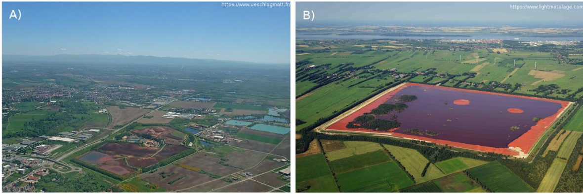
Figure 9. A) Tailings dump of residual red gypsum at the Ochsenfeld site, Eastern France; B) Red mud tailings pond at the Aluminium-Oxide Stade GmbH plant in Stade, Germany.
