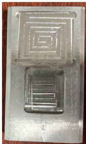
Figure 2.5 Stainless steel sample holder.
