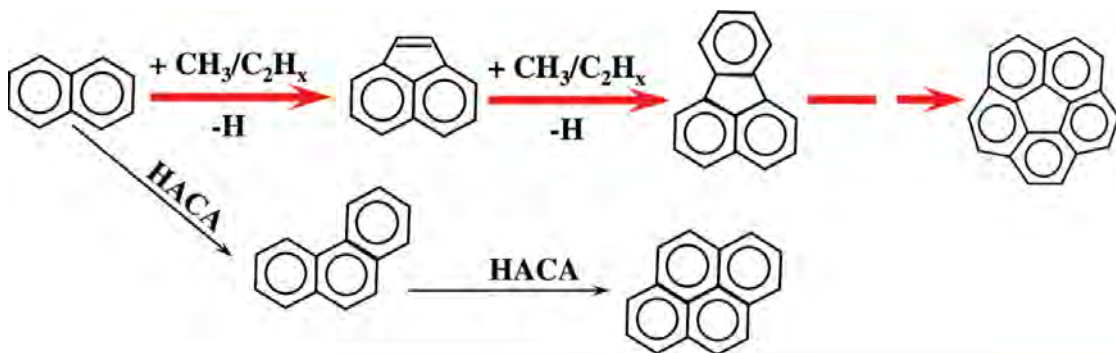
Figure 1.6 Presentation of the HACA and HAVA processes in the growth of PAHs from naphthalene. The red arrow means that HACA, HAVA and MAC can be involved. From Shukla and Koshi [2012a].
