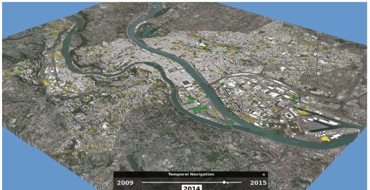
Figure 3.12.: Screenshot of the visualization of the city of Lyon in 2014 in UD-Viz , using 3D Tiles extended with 3DTiles_temporal .
