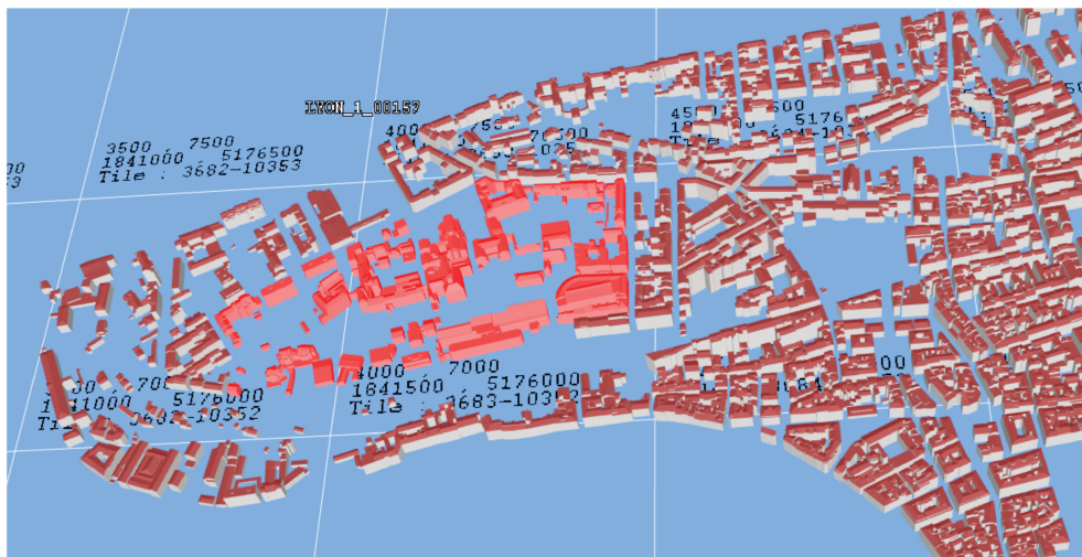
Figure 5.2.: Screenshot of a borough of Lyon 2009 vintage. In red, a building as defined in the CityGML file, which corresponds to multiple buildings in the real world.
