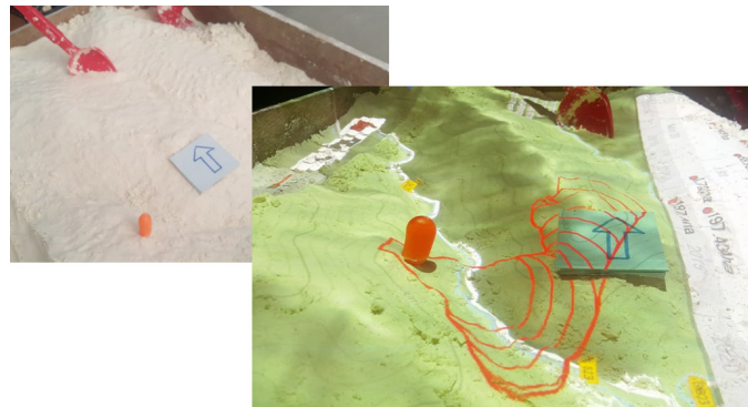
Figure 2.1: An AR Sandbox (left) shows a FireCasterAPI simulation (right) once illuminated with interactive video-projector
