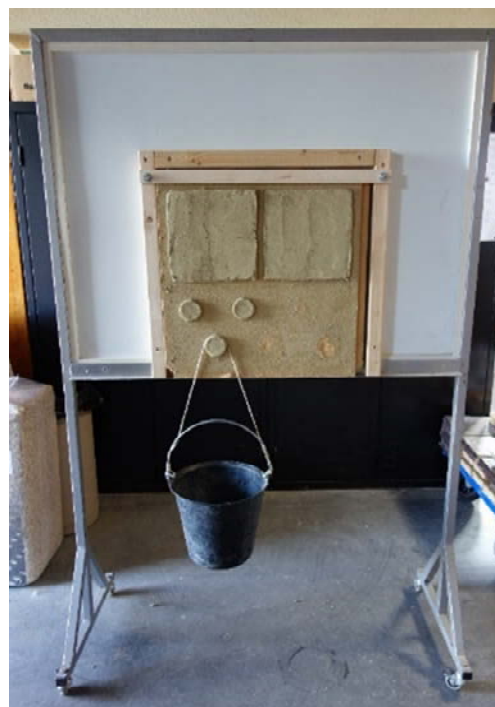
Figure 3.22. Shear test assembly.
