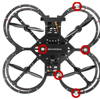
Figure 1.12 – Markers used for location
