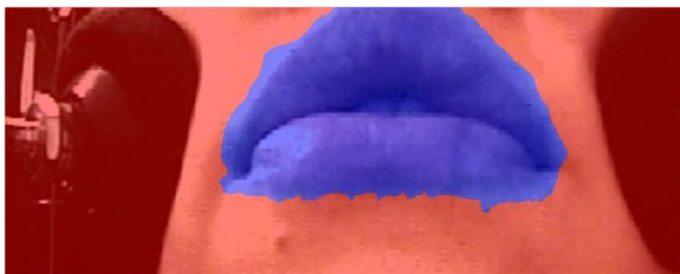
Figure 5.4: Automatic segmentation of the mouth (in blue) via semantic segmentation using a CNN.
