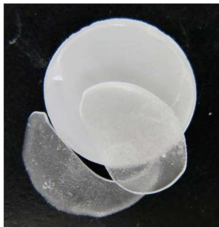
**Fig. 1 – Fractured VM7 sample.**
