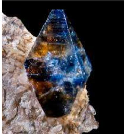
Figure 13 : Forme QUADRATIQUE : cristal d'anatase ( $\text{TiO}_2$ ) (source : <https://www.sciencedirect.com/topics/chemical-engineering/titanium-dioxide>)
