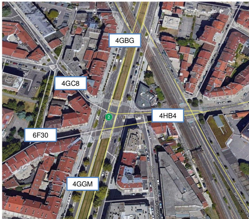
Figure 5.9: Location of BT devices around intersection 2, with their corresponding ID in database.
