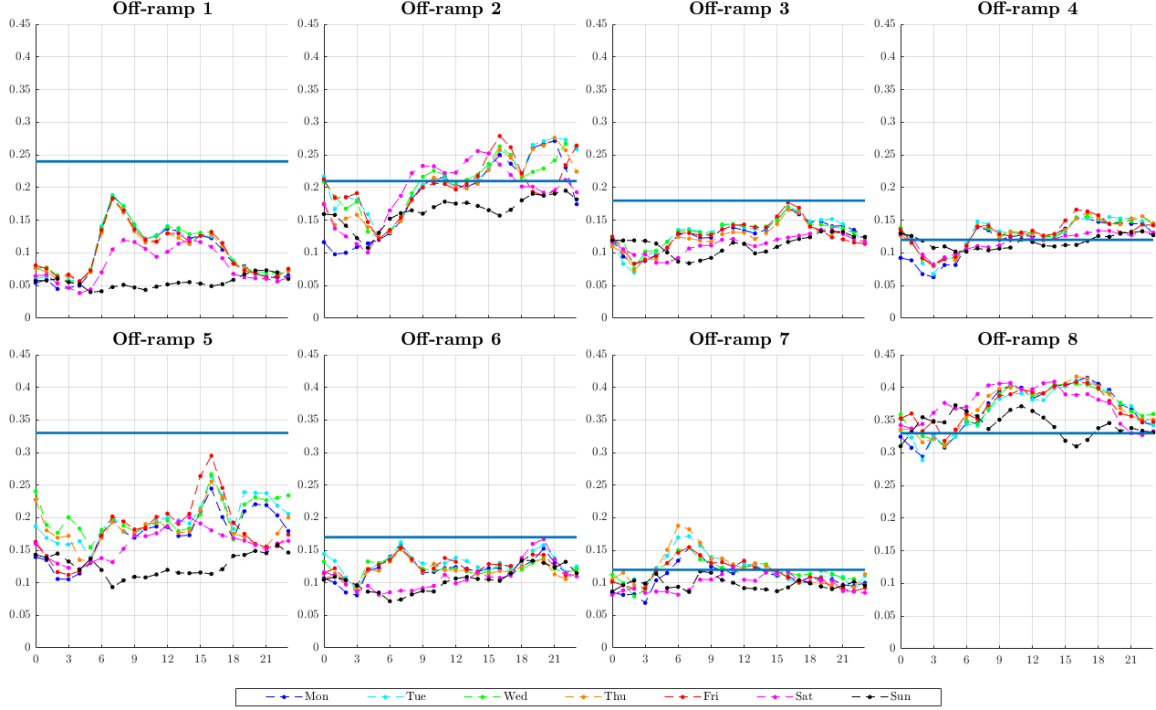
Figure B.4: Time series of the measured TRs for the days of the week for each intersection. For intersection 8 only the right turn ratio is shown.
