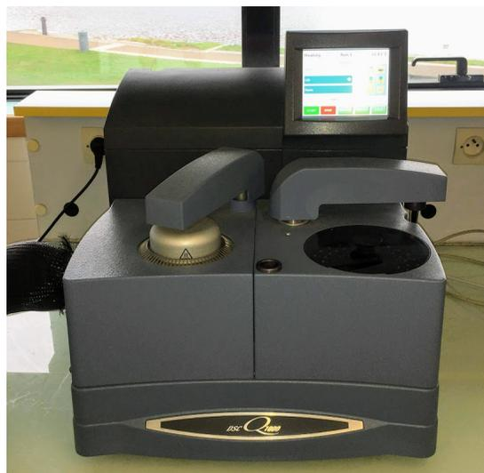
FIGURE 3.33 – Dispositif de type DSC model TA Instruments Q1000.
