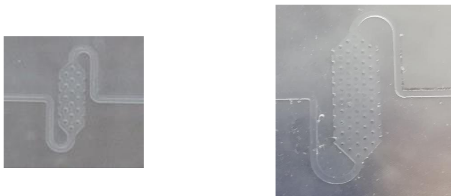
Figure 77: Photos of the small volume 1.32 \mu\text{L} pillar based reservoir (left) and the bigger one that can be compared to the serpentine reservoir (right) that can contain 17.3 \mu\text{L} .
