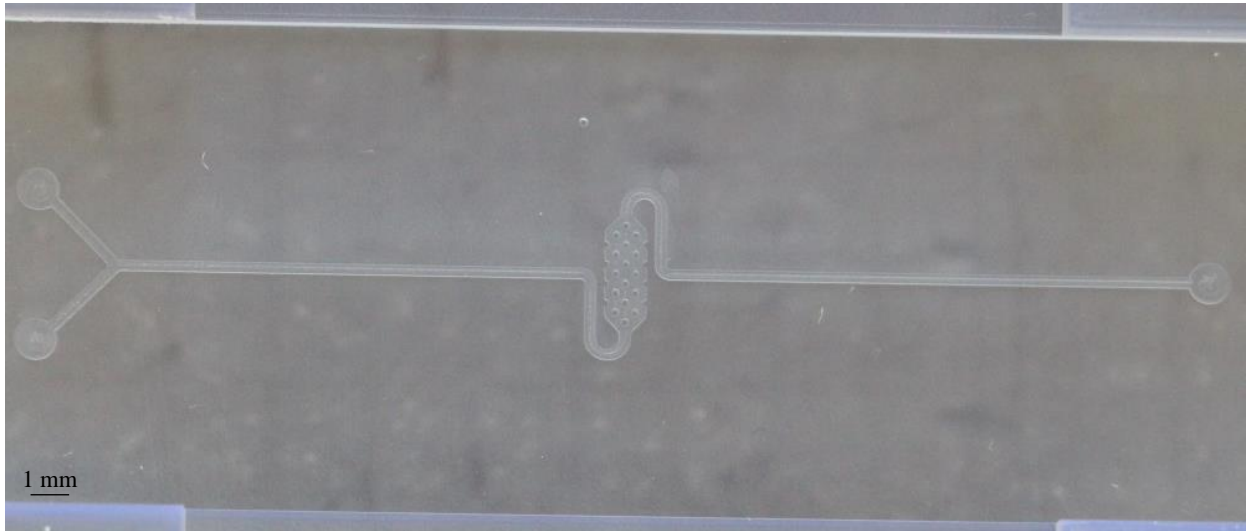
Figure 74: Pillar based reservoir. (Above) Openscad design. (Below) Photo of the realized pillar master mold.
