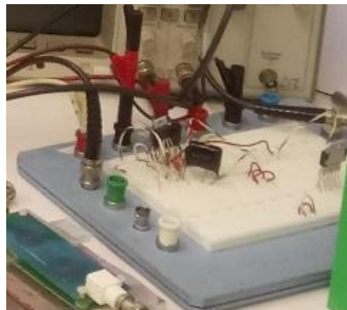
Figure 41: Voltage amplifier tested using a Labdec board.
