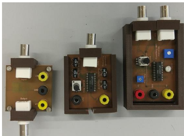
Figure 42: First trails of miniaturization of low frequency electronic parts. (a) voltage amplifier, (b) is a low frequency generator using a VCO and (c) is the first version of a combined VCO and amplifier.
