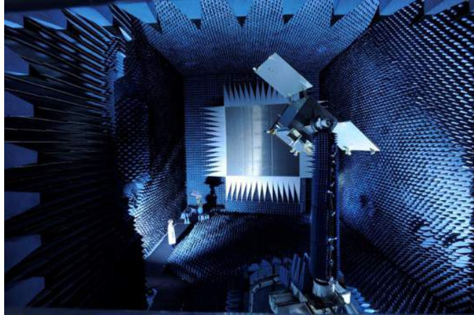
Figure I.9: CATR measurement at CNES with a serrated reflector. Credits: D. Belot, CNES.
