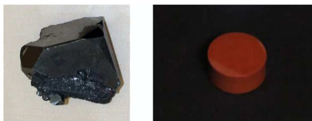
Figure 15. Samples of hematite crystal (left) and the hematite-epoxy composite material (right) with 10% of volume fraction of hematite nanocubes in the resin.
