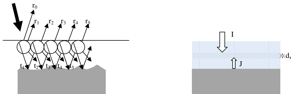
Figure 3. Schematic descriptions of two phenomenological models for multiple scattering of light; Melamed model (left) and the two flux Kubelka-Munk model (right)
