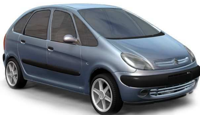
Figure 8. A car virtually painted by using a measured spectral BRDF 5 . Limited precomputed spectral radiance transfer is achieved by convolving the BRDF by the HDR sky (rescaled to D65 spectrum). Final image rendered by fast scan line algorithm. The other material models (for plastic, glass, etc) remain believable (not predictive).
