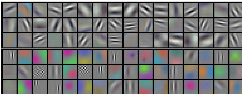
FIGURE 2.2: 96 convolutional kernels of size 3@11 \times 11 learned by the first convolutional layer on the 3@224 \times 224 input images by AlexNet. Reproduced from (Krizhevsky et al., 2012).
