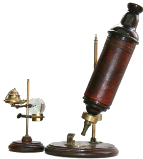
(a) Microscope manufactured by Christopher White of London for Robert Hooke. Hooke is believed to have used this microscope for the observations that formed the basis of Micrographia
