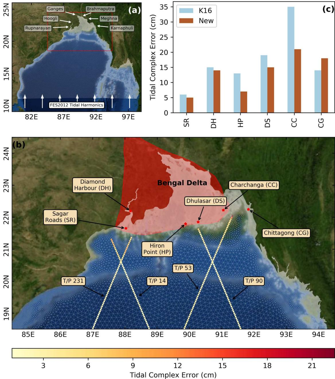
Figure 3.9: (a) Model mesh over the domain with indication of the open boundary conditions used. (b) A close-up of the model mesh over the study area. The tidal complex error is shown in colour-scale along the satellite altimetry tracks. The coastal tide gauges used for validation are shown by red stars. The Bengal delta is shown in red translucent patch (c) Bar plot showing the tidal complex error compared to Krien et al. (2016) (denoted as K16) for the 6 tide gauges shown on (b).
