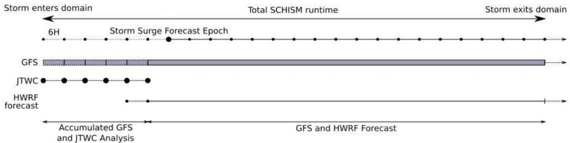
Figure 5.6: Temporal combination scheme of the JTWC, GFS, and HWRF forecasts for each 6-hourly storm surge forecast epoch.
