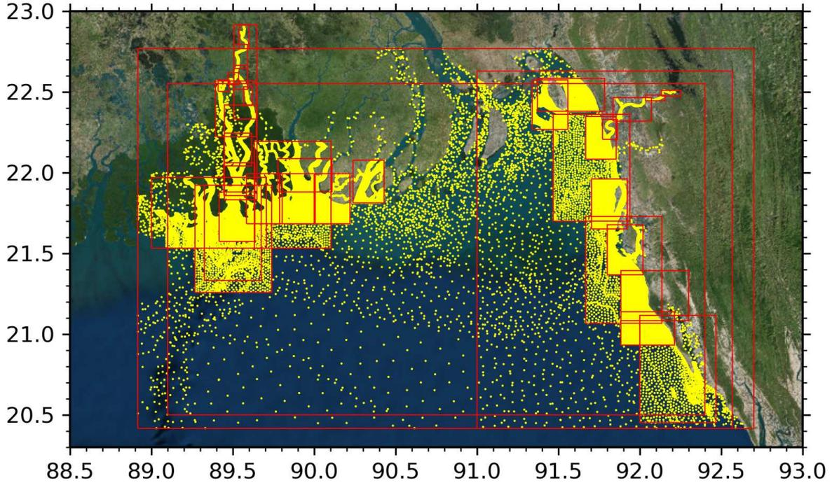
Figure 2.1: 77000 digitized sounding points (in yellow). The coverage of the corresponding individual charts is shown in red outlines.
