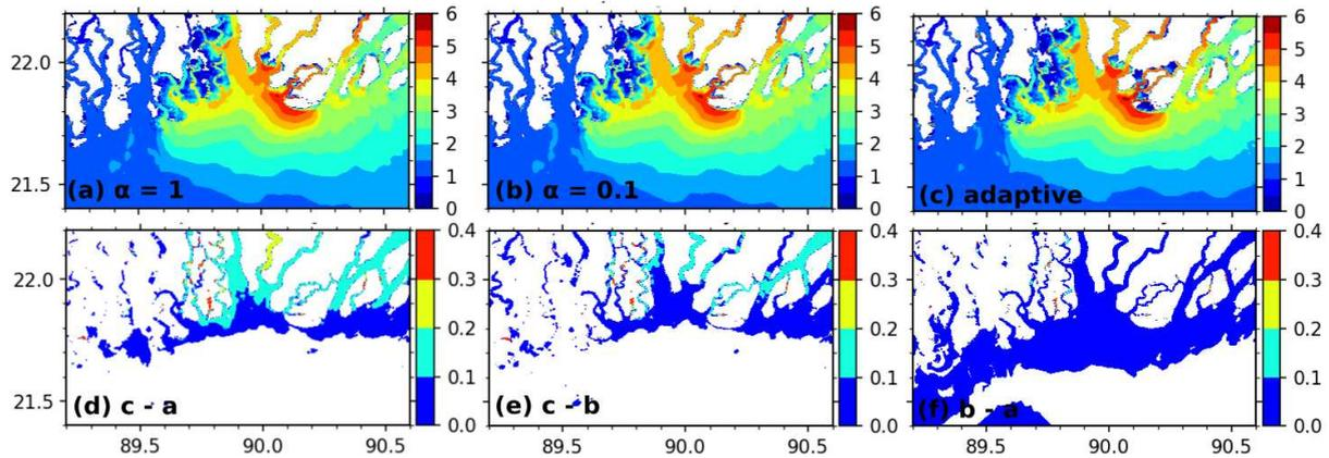
Figure 7.2: Maximum modelled water level during cyclone Sidr with (a) default wave breaking parameterization ( $\alpha=1$ ), (b) the parameterization used in this study ( $\alpha=0.1$ ), and (c) adaptive parameterization proposed by (Pezerat et al., Accepted). (d) and (e) shows the maximum water level difference between adaptive and  $\alpha = 1$  and  $\alpha = 0.1$  respectively. (f) shows the maximum water level difference between  $\alpha = 0.1$  and  $\alpha = 1$ .
