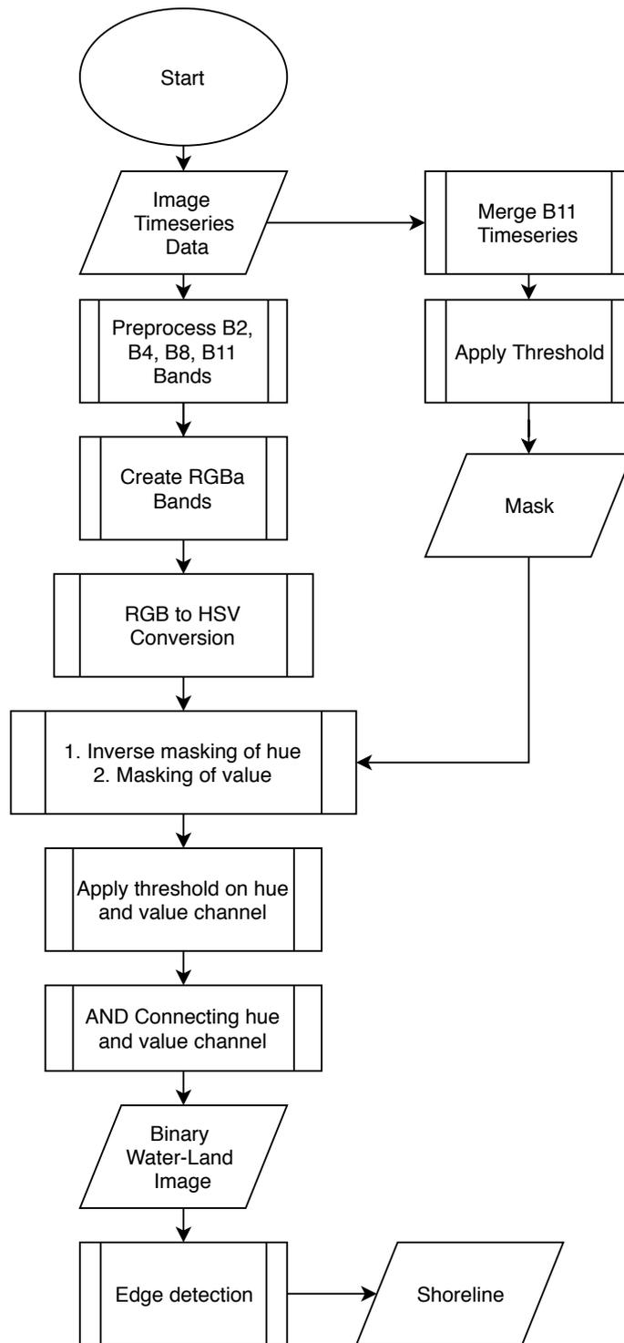
Figure 3.8: Flowchart of the shoreline detection procedure.
