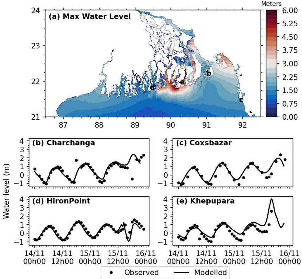
Figure 6.3: (a) Maximum simulated water level during cyclone Sidr. Comparison of simulated and observed water level during cyclone Sidr at (b) Charchanga, (c) Coxsbazar, (d) Hironpoint, and (e) Khepupara. The station locations are shown in (a).
