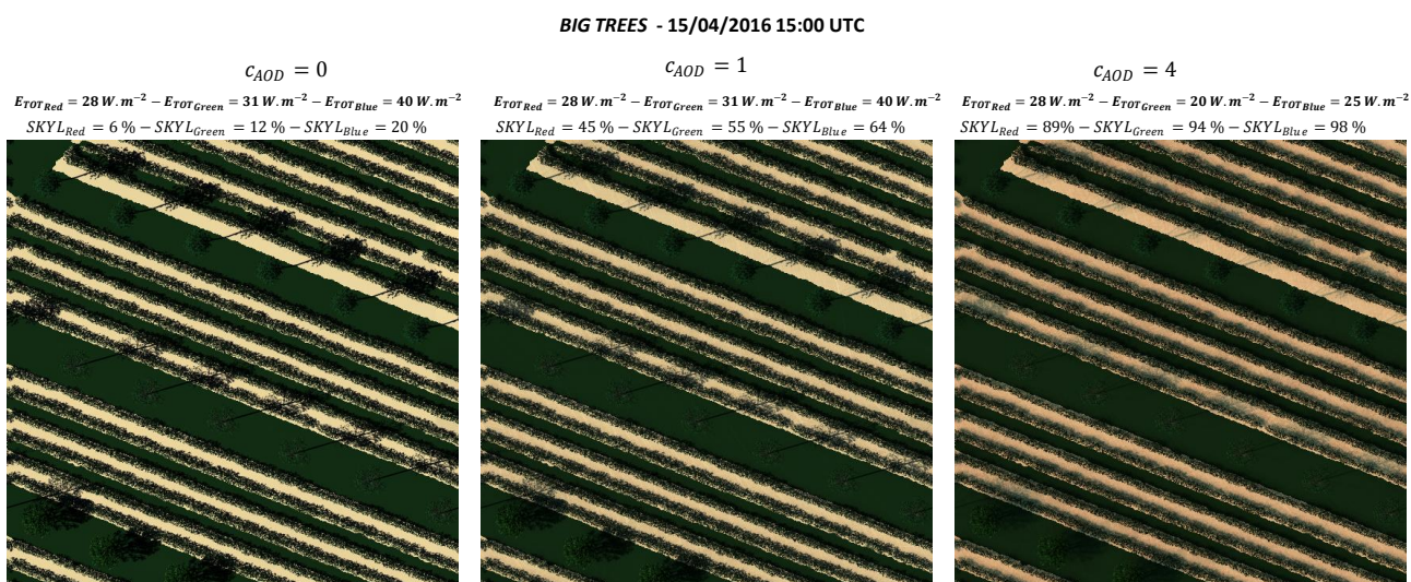
Figure 115: Visual check of the incidence of modifying the multiplicative factor of the Aerosol Optical Depth ( C_{AOD} ). Simulations of the RGB images were performed on the BIG TREES mock-ups of vineyards on 15/04/2016 15:00 UTC. The total irradiance ( E_{TOT} ) and the SKYL (diffuse to total irradiance ratio) are given per spectral band
