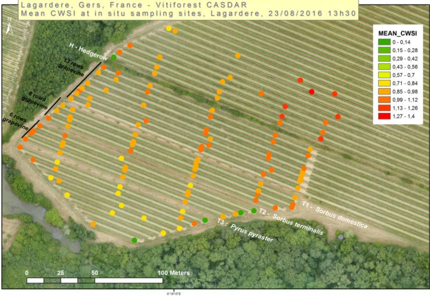
Figure 144: CWSI on 2016/08/23 – 13h 30 local time. The values correspond to the mean of vine pixels at plots of agronomic sampling, study site of Lagardère (32).
