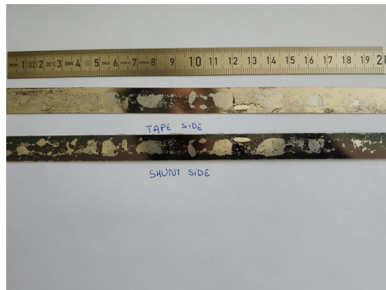
Figure 5.17: Fastgrid conductor manufactured with the industrial process. The sample was delaminated in purpose.
