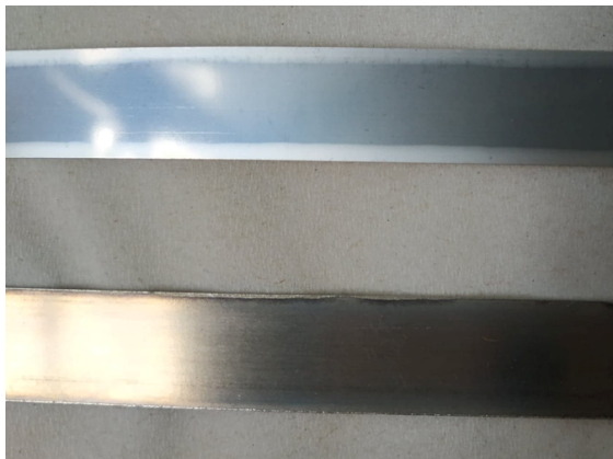
Figure 5.6: Picture of the bare tape from THEVA (top) and Fastgrid conductor (bottom).
