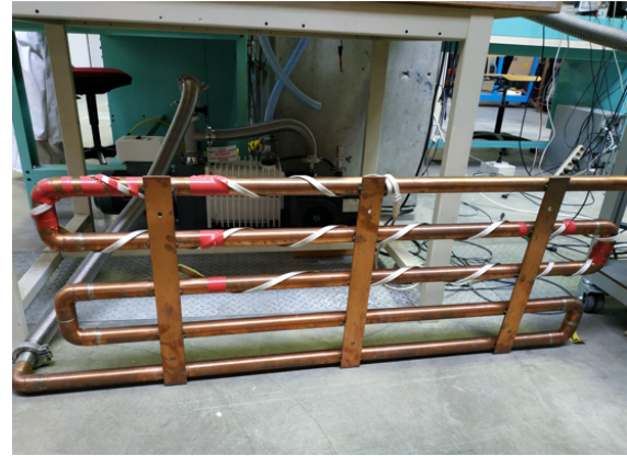
Figure 3.10: Picture of the experimental set-up used to decrease the pressure over the cryogenics bath: two pumps are associated in parallel (background) and connected to a heater (foreground).
