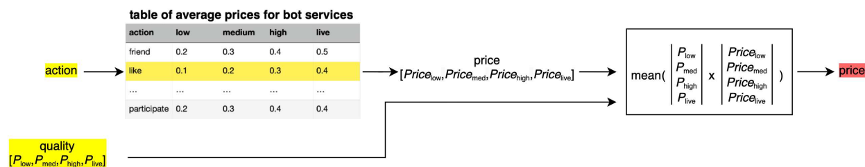
Figure 4.18: Technique for bot's price estimation. Inputs of modules are highlighted with yellow, and outputs with red.
