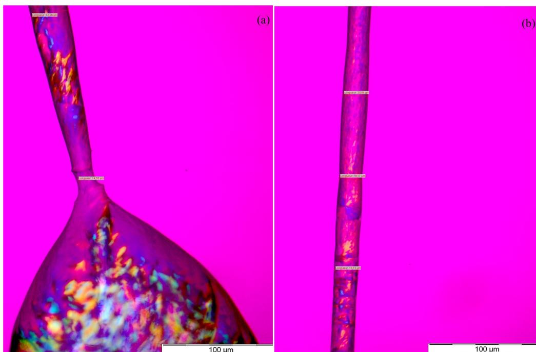
Fig. D.1 Beads-on-a-string (BOAS) microscopy for PEG20PEO1000, obtained from the Polarised Light Microscopy. (a) The view around the neck. The size of the big drop is  $\approx 220 \mu\text{m}$  and the size of the pinching point is  $\approx 14 \mu\text{m}$ . (b) The view of the filament, connecting different beads, and the average diameter  $\approx 20 \mu\text{m}$  can be observed.
