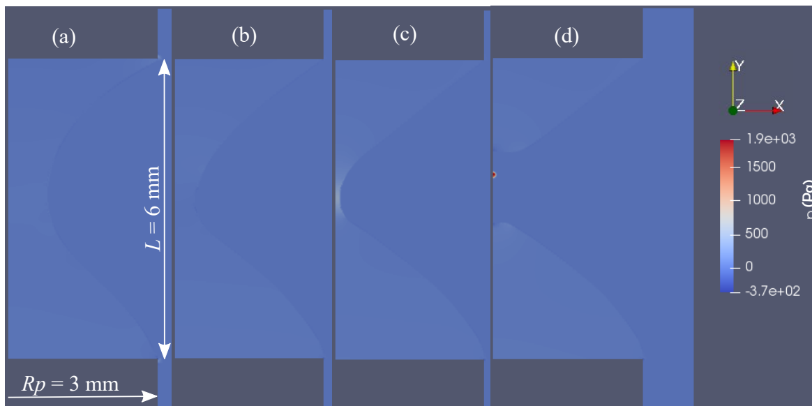
Fig. 2.18 Visualisation of pressure, p (Pa), inside stretched liquid bridge for PEG20PEO1000 solution using Mesh N3. In these simulations, we used: R_p = 3 mm, FAR = 2 , De = 132.8 and Oh = 1.84 . Pressure, p (Pa), at (a) t = 0 , (b) t = 0.020 , (c) t = 0.027 , and (d) t = 0.029 s.
