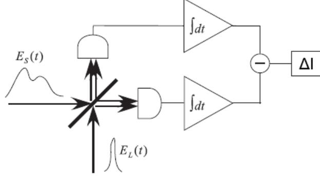
Figure 2.2: Homodyne detection setup (from Ref [14]).
