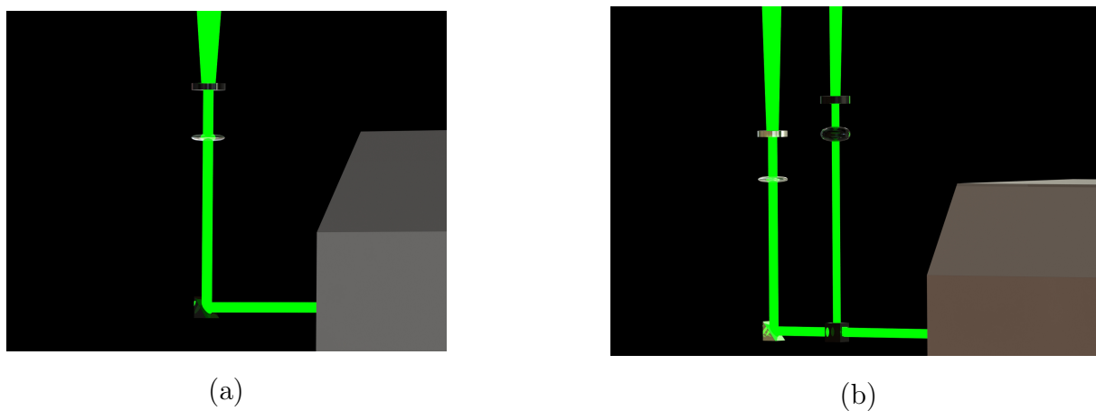
Figure 5.4: Sketch photographs of the laser beam direction and the optics that are used for the corresponding set-ups: (a) a corner mirror, a spherical focal and a cylindrical focal direct the laser sheet parallel to the leading edge (1st set-up). (b) The laser beam is split in two and finally two laser sheets cross the flat plate vertically. One corner mirror, one spherical, one cylindrical focal and one splitter are used for directing the laser sheet (2nd set-up).
