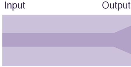
**Figure 2.8** – Waveguide with large taper at the output facet.
