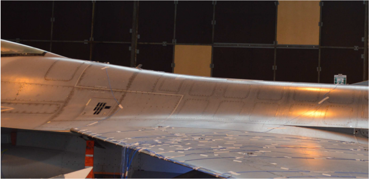
Figure 3: Dynamic strain sensors on the ground vibration testing of an F-16 aircraft, illustrating the coarse measurement point density on a large-scale test. Extracted from [ dos Santos et al. 2015 ].
