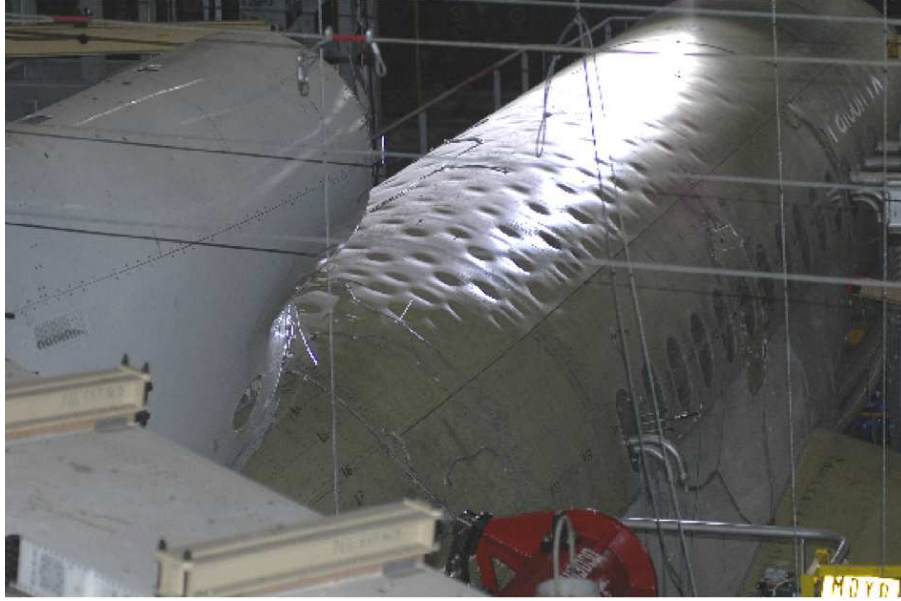
Figure 4: Falcon 7X fuselage local buckling during static tests. Figure reproduced from [Barrière 2014].
