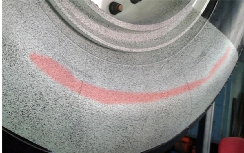
Figure 7.11: Specular reflection appearing on SDIC images of an airplane tyre sidewall during experiments mimicking the tyre/runway interaction. Courtesy of DGA Aeronautical Systems.
