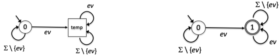
FIGURE 6.1 – Automates after ev temp (gauche), et before ev trace ou trace until ev (droite)
