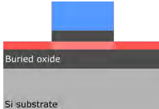
Figure I - 4. Schematic representation of an SOI device with a fully depleted channel.
