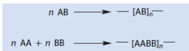
Figure 15: Schematic representation of the step-growth polymerization of AB-monomers and AA/BB monomers. Adapted from Koltzenburg et al. 135
