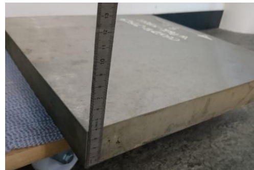
Figure 51 –Sample of SS316L(N)-IG plate 400x400x40 mm 3
