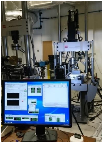
Figure 49 – MTS-322 Traction-compression machine
