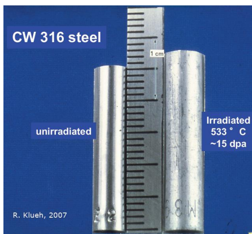
Figure 39 – Swelling (effect of vacancy clustering) of CW 316 steel (Klueh, 2008).
