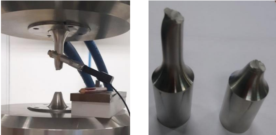
Figure 67 – Cylinder 03 after failure
