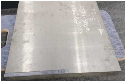
Figure 51 –Sample of SS316L(N)-IG plate 400x400x40 mm 3
