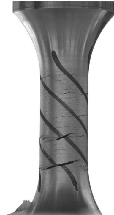
Figure 98 – Cylinder 11 after 42183 cycles
