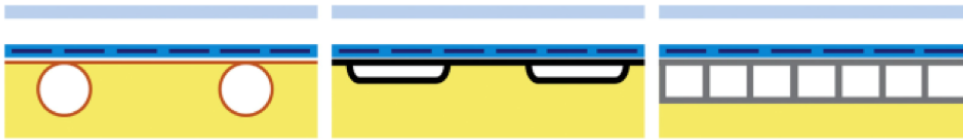
FIGURE 2.22: Tubular, trapezoidal and rectangular channel collector [28]
