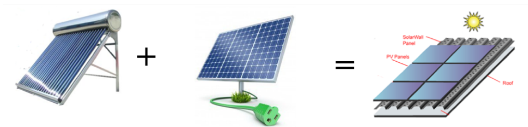
FIGURE 2.11: Schematic diagram of PVT components
