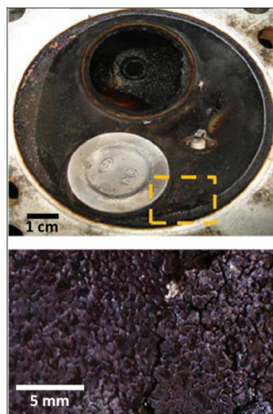
Figure 7: Enlarged image of cylinder-head deposits [38].
