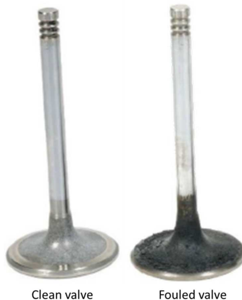
Figure 5: Comparison of a clean intake valve and a fouled intake valve [33].
