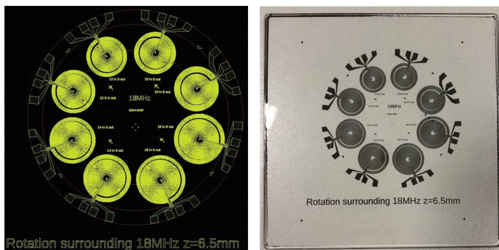
Figure 2.8: The left image represents the design for the transducers using layout editor software. The right image presents the optical mask of the design.
