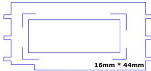
Figure 2.13: Design of the frame to be cut.
