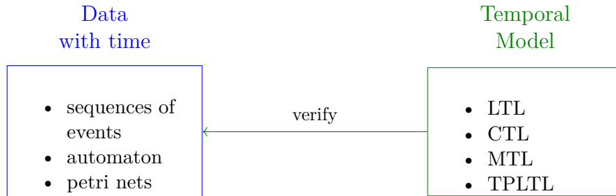
Figure 2.4 – Model checking to query sequences of events or DES
