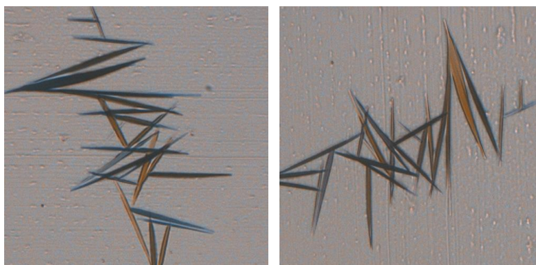
Figure V. 29 Needle type crystals of HDPPD grown upon exposure to vapor of chloroform.
