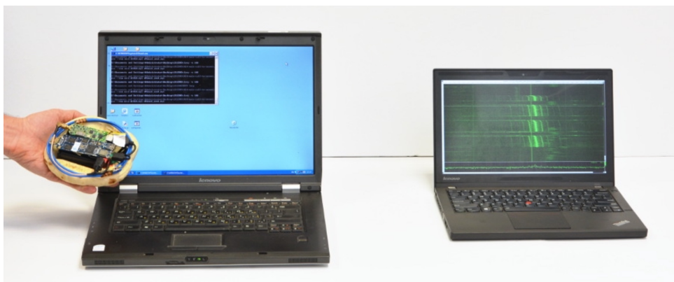
Figure 1.9 – The Pita handheld prototype measures the target computer (left) at a specific frequency band and streams the digitized signal over Wi-Fi, in real time, to the attacker's computer (right).
