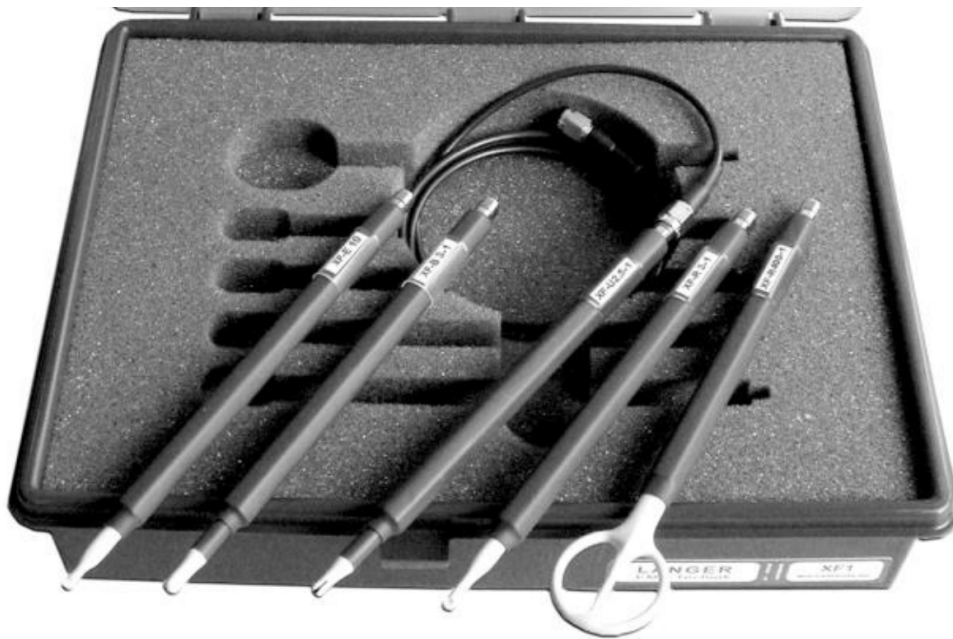
Figure 1.7 – Near field probe set of 4 Langer H-field probes (left) and one E-field probe (right).
