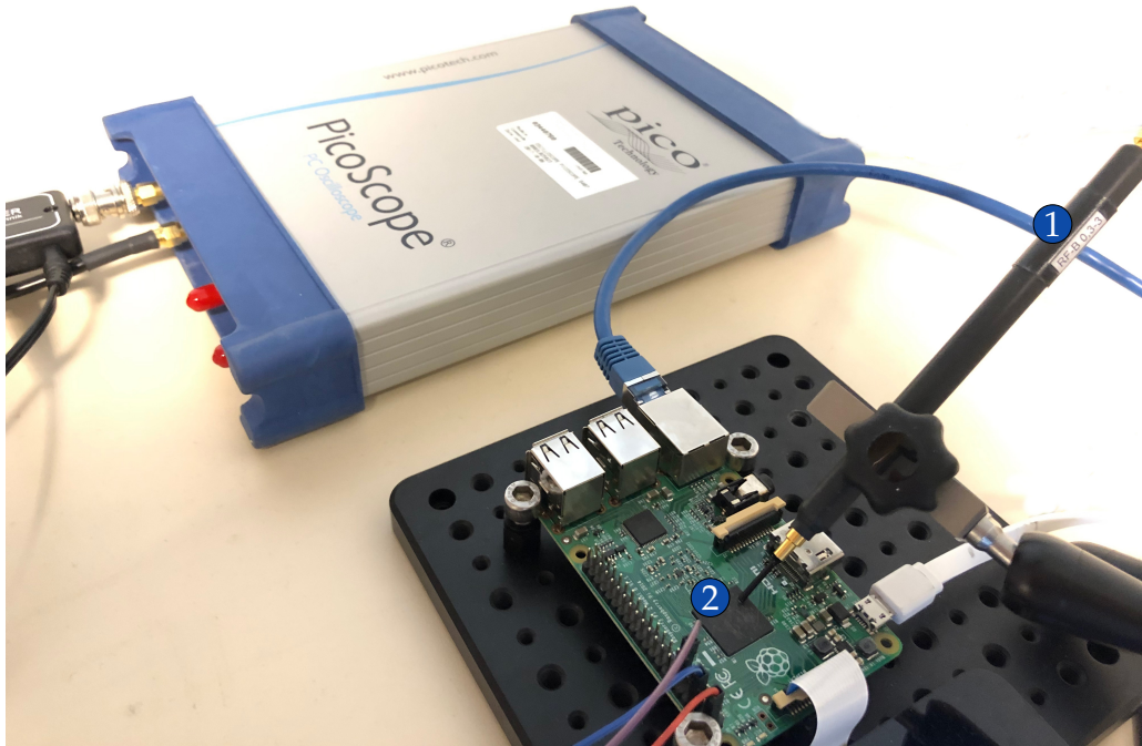
Figure 3.4 – Probe setup consists of a H-Field probe ① placed 45 degree above the Raspberry Pi processor ②.
