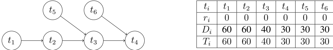
Figure 6.7: An instance of 6 periodic tasks and the associated DAG \mathcal{G} extracted from ROSACE case study [41].
