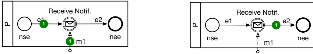
Figure 4.23: Starting Behaviour of a Catching Message Intermediate Event. Before (left) and after (right) application of the St rule.
