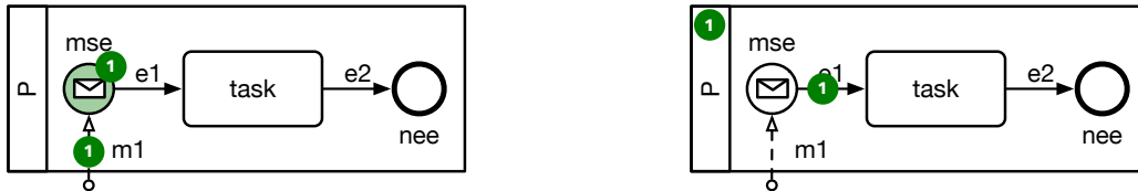
Figure 4.11: Completing Behaviour of a Message Start Event. Before (left) and after (right) application of the Ct rule.
