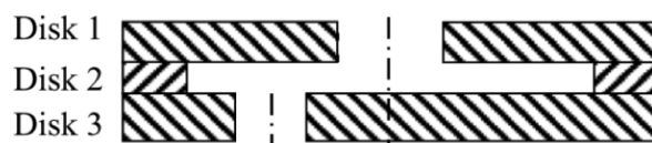
Figure 4.1: Compound nozzle geometry: triple-disk injector.
