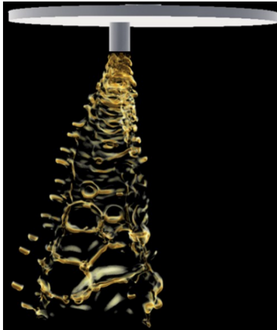
Figure 6.12: Volume rendering of the atomizing jet issued from a low-pressure compound nozzle.
