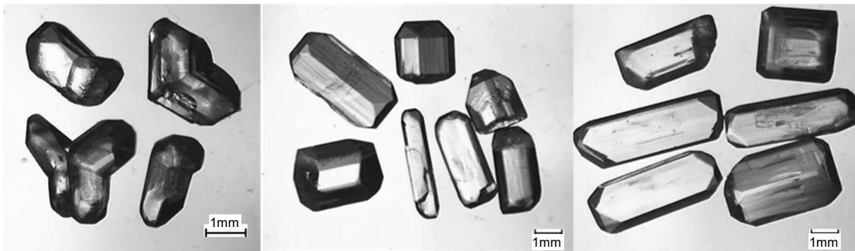
Figure 4-8-K 2 SO 4 crystals obtained from supersaturated solutions \beta=1.25 : typical twin crystals observed in this study (left), crystals obtained by laser irradiation (middle) and crystals obtained by spontaneous nucleation (right). Pictures taken with a NIKON SMZ-10A microscope equipped with a Sony DXC-950 3CCD Color Video Camera Power HAD
