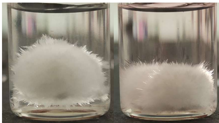
Figure A-10-Pictures of the DPL crystals obtained in 1mL vial, on the left aqueous solution and on the right gold doped aqueous solution.
