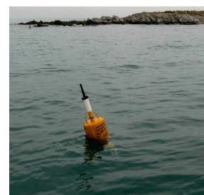
(c) SAMBAT probe installed near surface.
