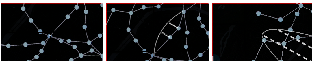
Figure 3.5: Close-up of SlidingElastic (combined view). From left to right: when moving away from the selected subpath, a curved copy of the path follows the user, even if the path is no longer in the HoloLens view. Again the view is the combination of the shared wall display view (graph) and the head-mounted display (elastic path and its connections only).
