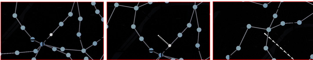
Figure 3.4: Close-up of SlidingRing (combined view). From left to right: as the user moves its field of view away from the link the ring is attached to, the trail (dashed line) guides the viewer back to the link, even when the ring is no longer in the AR view (right).
