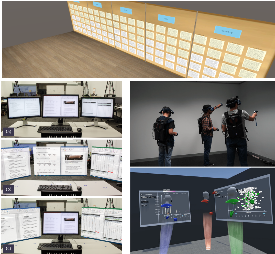
Figure 2.3: Alternative screen missing figures: on top replacing a wall display by a VR HMD application [132], on bottom left, replacing additional desktop screen in AR [163], on bottom right, replacing large displays by VR HMDs [124]
