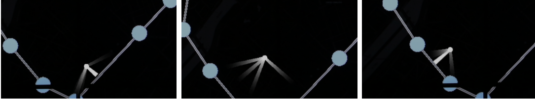
Figure 3.7: Close-up of MagneticArea. From left to right: the magnet is attached to a link (on the wall display); as the gaze-cursor moves other link candidates are drawn to it and attraction lines become more visible; until the magnet detaches and reattaches to another link.
