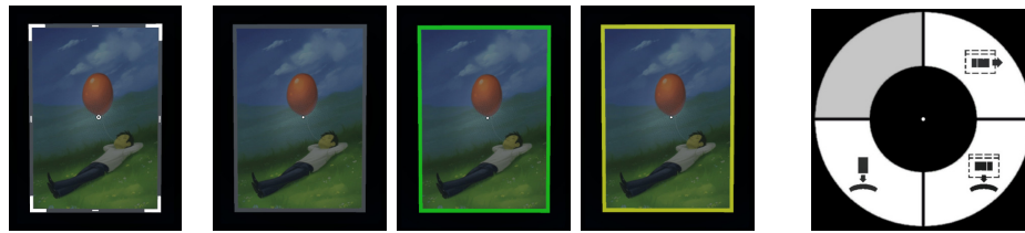
Figure 4.3: Visual feedback on the cards and menus, all rendered either on the wall or in AR. On the left: the focus highlight that is added in AR to the card when the user gazes at it (personal content not seen by others). In the middle, the Card selection states, visible by all users: the card in its initial unselected state; the card selected by a user who is assigned the green color; and by the user who is assigned yellow. The last image shows our contextual menu, only visible to the user that invokes it. In this case, the contextual menu has been invoked on a card that exists on a virtual surface, so we see the available options to move the card to the Personal Space , to move all content of the surface towards another surface, or all content towards the Personal Space .
