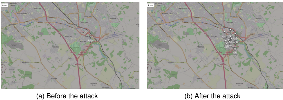
Figure 2.6: Simulated Ghost Aircraft Flooding attack showing the appearance of multiple ghost aircraft to confuse air traffic controllers and pilots.
