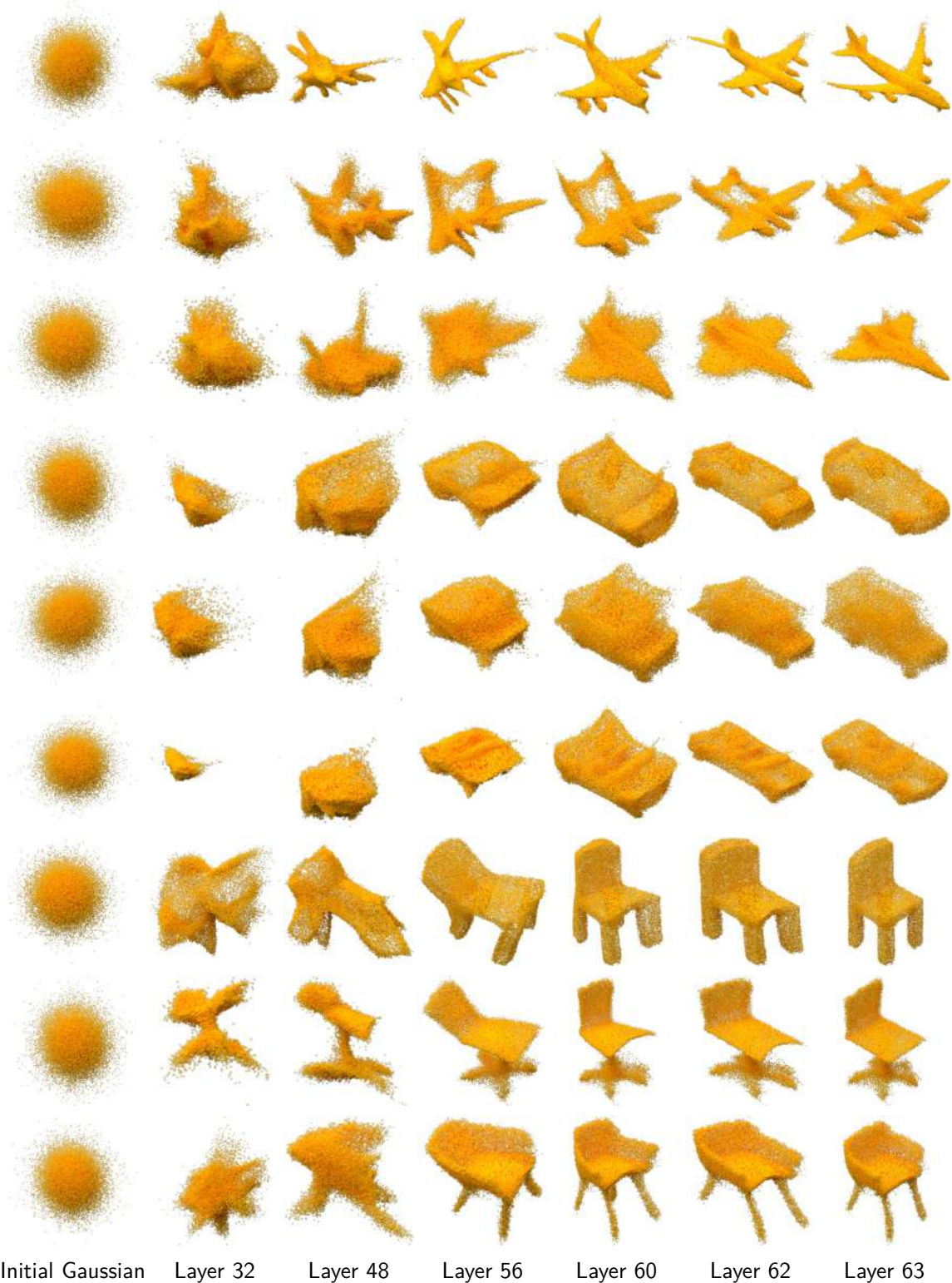
Figure 4.6: Evolution of points in reconstructed samples across different layers of the flow in DPF-Networks. For each sample we generated 32,768 points.
