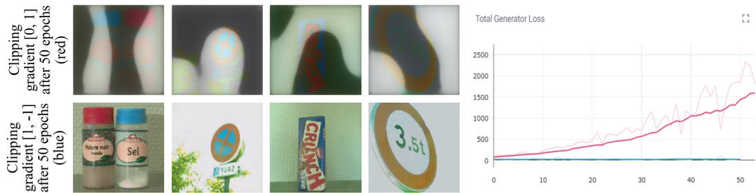
Figure 4.20: Ablation study (after 50 epochs) of clipping gradients before backpropagating weights. Clipping the gradients to  $[0, 1]$  resulting in exponentially increase in the generator loss and produced poor resulting images.
