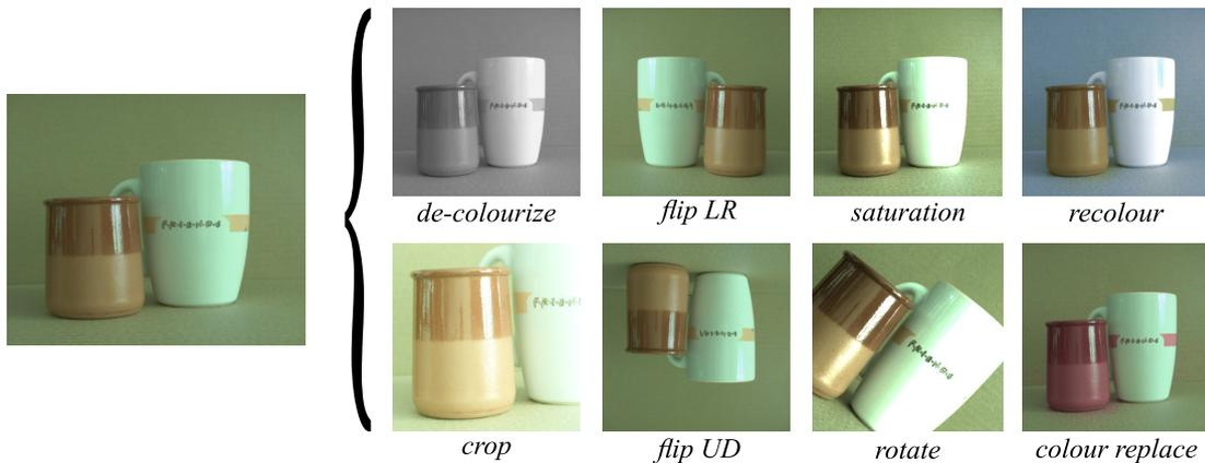
Figure A.7: Example of various non-destructive and destructive transformations for data augmentation that can be used for increasing the dataset size without causing the network to overfitting trained weights.
