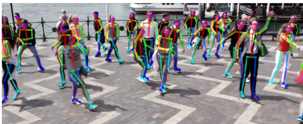
Figure 1.5: 2D pose estimation by OpenPose [Cao2019].
