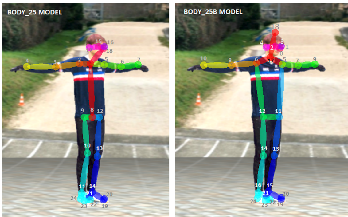
Figure 2.7: The body_25b OpenPose model is more accurate than the default body_25 one. As an example, the left knee is slightly misplaced on the default model. Keypoint definition and order also differ between both models.
